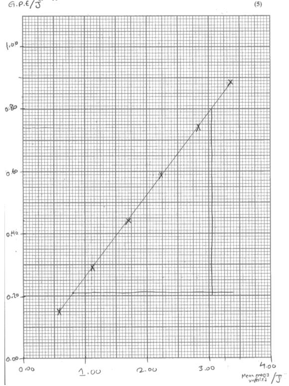
This is an example of a graph that was awarded 5 marks. The axes are labelled correctly, the scale increases by 0.1 per 2 cm on the *y*-axis and 0.5 per 2 cm on the *x*-axis, the plots are within 2 mm and the line is straight and balanced (with 2 points above and 2 points below the line).
